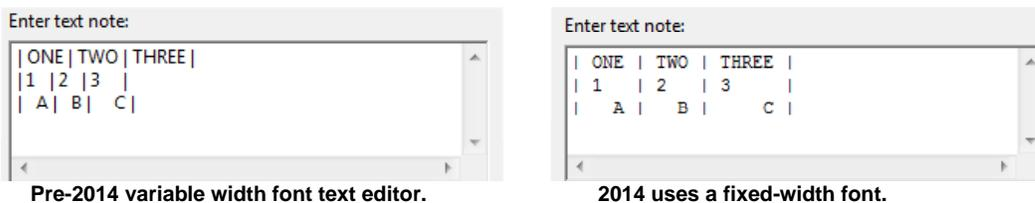
By default, the fixed-width font Courier New is used for text edit controls. This font can be modified by setting the text buffer `PANEL_TEXTEDITOR_FONT` to the font of your choosing in your `ExpertCAD.cfg` file.
