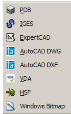
AutoCAD DXF and DWG output is a new feature for 2009. Both options respond to the 2D Drawing Export settings in the Import/Export tab of the Tools/Options dialog.
